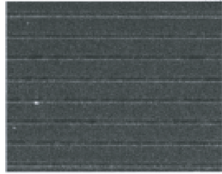
Fig. 3. Scanning Electron Micrograph of the magnetic grating G2 (see text) of period \Lambda = 1.8 \mu\text{m} and width w = 1.5 \mu\text{m} .
